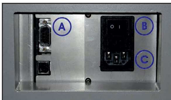
Fig. 2 Connector Terminal on the Backside of the Instrument. (A) Barcode Reader; (B) Power Switch, and the (C) Power Cord.
