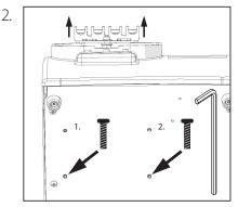
The tube carriage will slide back. Lift the tube carriage to align the motor mount holes to the holes in the base plate.
