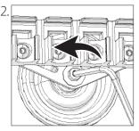
Use the supplied 3 mm allen wrench to loosen the central screw and remove restriction tie and old neck gasket.
