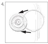
Secure the new neck gasket using the restriction tie with the clamp positioned toward the bottom of the instrument. Tighten central screw.
