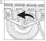
Use the supplied 3 mm allen wrench to loosen tube carriage holder screw
