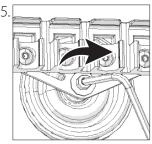
Use the supplied 3 mm allen wrench to tighten the central screw and secure the tube carriage.
