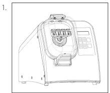
Remove all tubes, cover the unit in its plastic bag.
