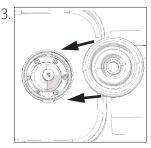
Slide the new neck gasket onto the pivot shaft and housing
