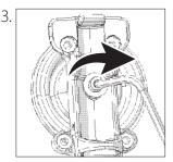
Use the supplied 3 mm allen wrench to tighten tube carriage holder screw
